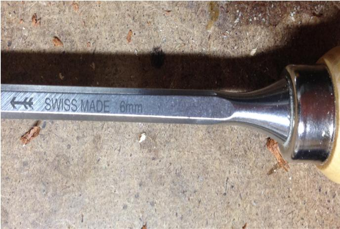
The one-eighth chisel was purchased recently to clear out a nut slot in a Fender-style neck. It worked great. The third chisel has the words “Swiss-Made” stamped. This is the mystery chisel. I do not remember how I came to be in possession of it. However, it’s a good one – I tested it on some hardwood and it cut very well. It’s a 6mm chisel (about one-fourth of an inch). It stands ready for whatever guitar or other hobby task that I can come up with.
