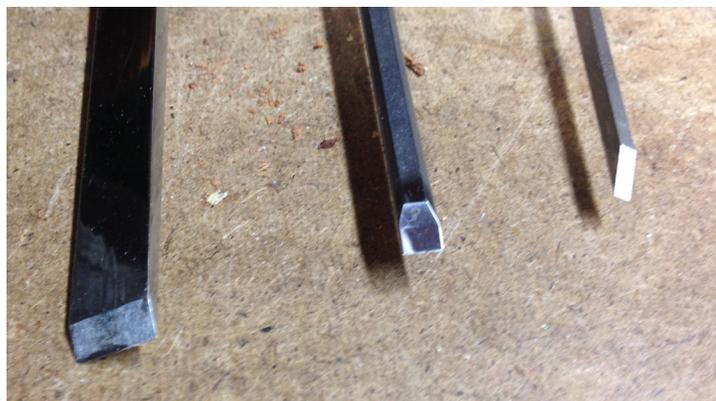
They are pictured at the beginning of this article. The business ends of the chisels are shown at the picture at the end of the left column. They are, from left, the LMII chisel; a "Swiss-made" chisel that I can't remember buying; and the one-eighth inch chisel I bought to clear out a nut slot in a Fender-style neck. (See the article "Better Lucky Than Good.")
