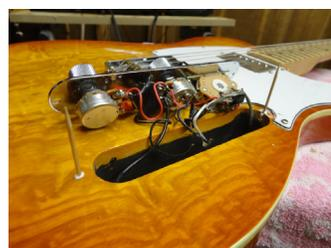
wiring looks messy. Maybe I can fix that, too. Notice the toothpicks glued into each screw hole. That should help with the screw problem.
