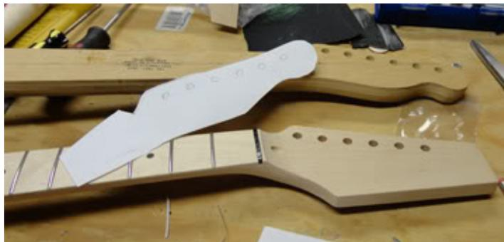
I used a combination of sawing and sanding with an oscillating sander to shape the neck. I was pleased with how it turned out.
