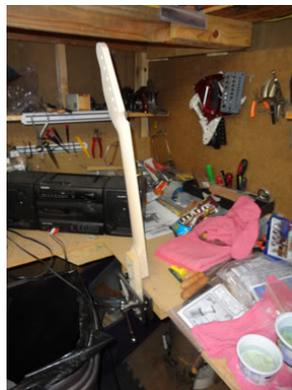
The neck attaches to the body with screws. The body already had holes for the screws.
