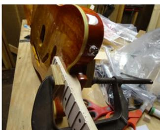
So, I clamped the neck and body together carefully. I used a cordless drill to go through the body holes and drill holes in the neck so it would be easier to drive in the screws.
