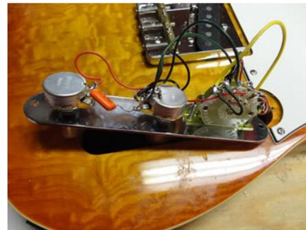
I used Alpha quarter-size pots. The switch was replaced with a CRL-type switch, similar to those used on higher-end Fender guitars and like the originals that were on the original Fender guitars. They
