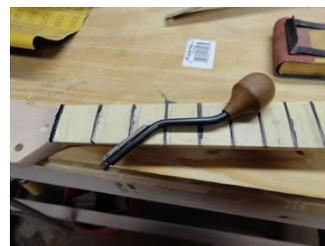
Now, after the frets are leveled, their tops are flat. This is not good. They should be rounded. That's what the fret rounding tool does. This baby is helpful especially when installing frets.
