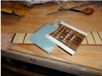
and can be used to polish the files after they are rounded, or "crowned."
